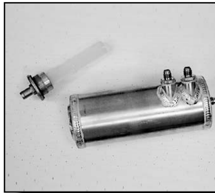
Fuel Accumulator Tank
